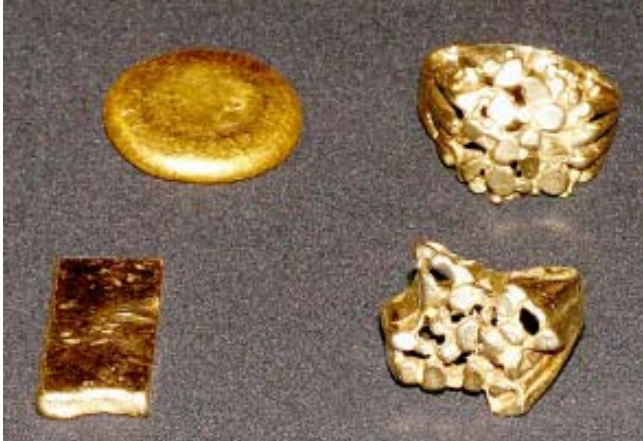
Clockwise from lower left: 14K ingot, 24K ingot, two 14K rings made from computer gold.
