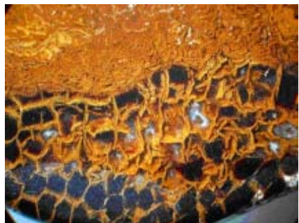
Figure 4: Microscope image of a hexagonally fractured specimen that shows the hexagonal pattern distorting and eventually collapsing in the upper half into a mass of orange agate. Magnification is about 6x.
